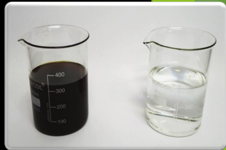
(Left) A feedstock blend of used cooking oil, corn oil and trap grease with a combined FFA of 65%. (Right) ASTM 6751, B100 after processing with Super TM process
